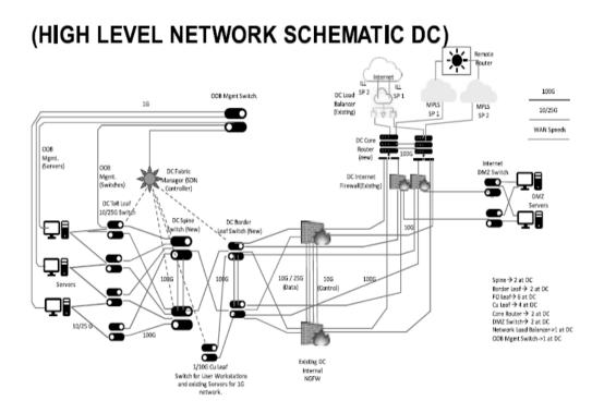
**6.** Present site network diagram is as below. The routers will be replaced with SDWAN boxes and switches with managed switches for site offices.
