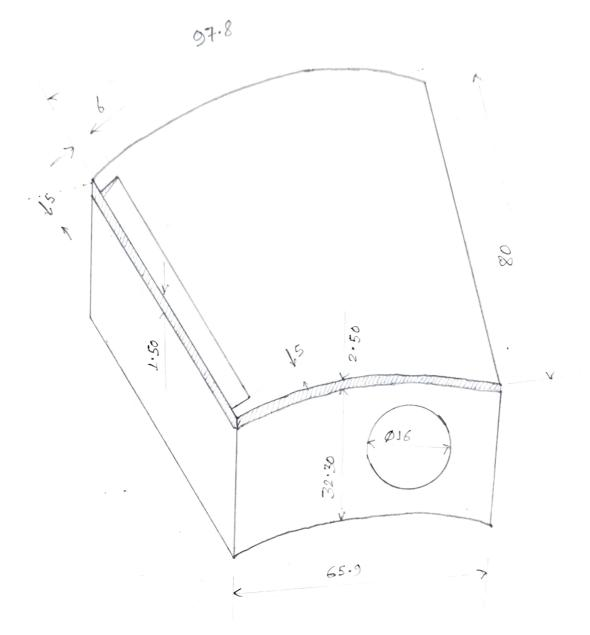
Thickness of flexible thrust pad (without babbit material)=32.30 mm
