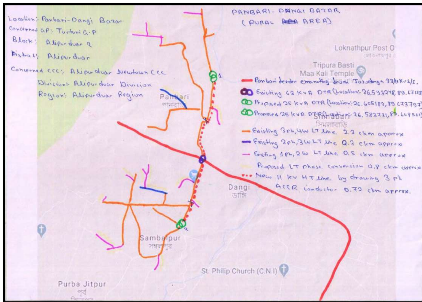
FIGURE 5.3: VIEW OF EXISTING HT/LT NETWORK OF SELECTED LOAD CENTRES FOR HVDS SUB-PROJECT AT ALIPURDUAR DISTRICT (AT PANBARI DANGI BAZAR 63kVA DTR UNDER PANBARI FEEDER)
