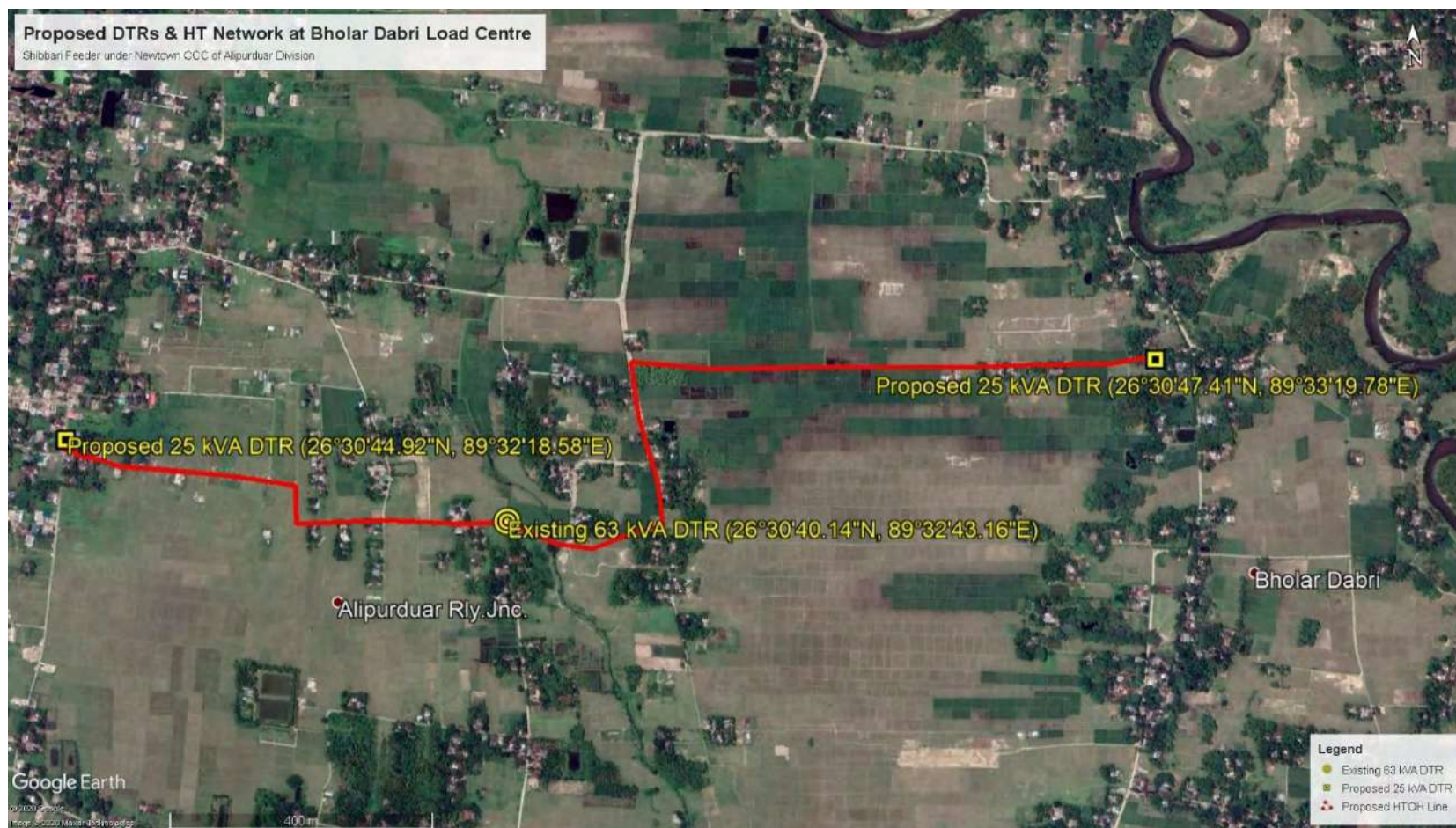
FIGURE 5.2: ENVIRONMENTAL & SOCIAL SETTING AT SELECTED LOAD CENTRES FOR HVDS SUB-PROJECT AT ALIPURDUAR DISTRICT (LOCATION OF PROPOSED DTRs & HT LINE :BHOLAR DABRI DTR(63kVA) UNDER SHIVBARI FEEDER)
